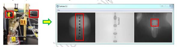
(12) Restore the latest QC workspace for 100um nozzle in "FCF QC Log" folder  $\rightarrow$  restore Laser Delay and Fluidics Setup. Load Rainbow beads and start running the sample  $\rightarrow$  Adjust the sample flow rate, sample pressure > sheath pressure 1psi  $\rightarrow$ Open Blue Laser shutter  $\rightarrow$  close the door in front of the nozzle and activate laser by presenting your finger onto the sensor.
