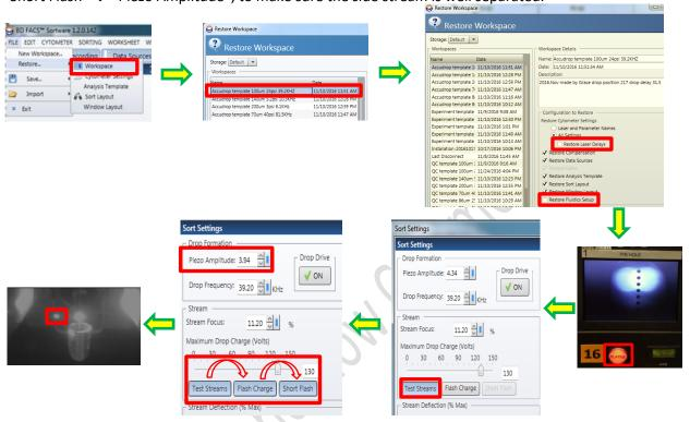
2. Load Accudrop beads → (17) turn the filter knob to Accudrop filter → run accudrop beads → click "Start" in the sort layout → adjust the "drop delay" until the left stream is as bright as possible while nearly no fluorescent signals can be detected in the mainstream. Change the Sort Mode to 1.0 Drop Pure and adjust the Drop Delay again → Turn the Accudrop filter knob back to the ND filter position.
