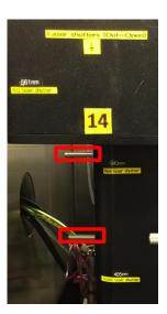
(15) Slightly adjust the horizontal knob to achieve highest signal strength and tightest CV. When all the alignments have been done, select QC Log folder to record FCS file → save workspace in FCF QC Log folder.
