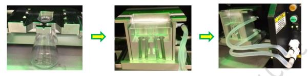
4. Restore a workspace for "Experiment" in Default folder→ charge deflection plates→double click "Test Stream" to adjust the position of the side streams → "Set Home".
