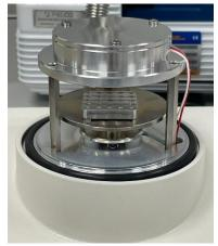
f) Cover the glow head with the glass chamber and center it on the o-ring. Check the setting on the screen and press "AUTORUN" if the setting is okay. The system default setting is as follow:
