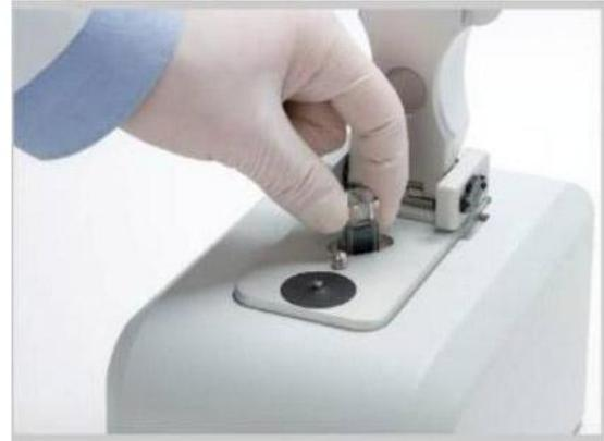
7. Lower the sampling arm and start measurement in the program. “Blank” Measurement is required before measuring the samples.
