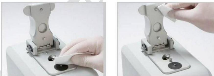
8. After all your measurement, add a drop of deionized water to the pedestal and clean with Kimwipe paper.
