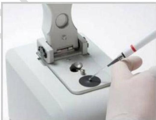
5. Lower the sampling arm and start measurement in the program. “Blank” Measurement is required before measuring the samples.
