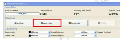
2.8 Go to **Normal Worksheet**, move the P1 gate to include major cluster. Adjust FSC and SSC PMT Voltage if needed.
