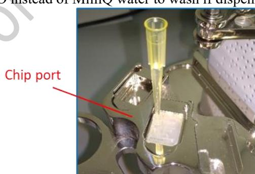
10. Select the chip from the chip port by clicking the corresponding chip number.
